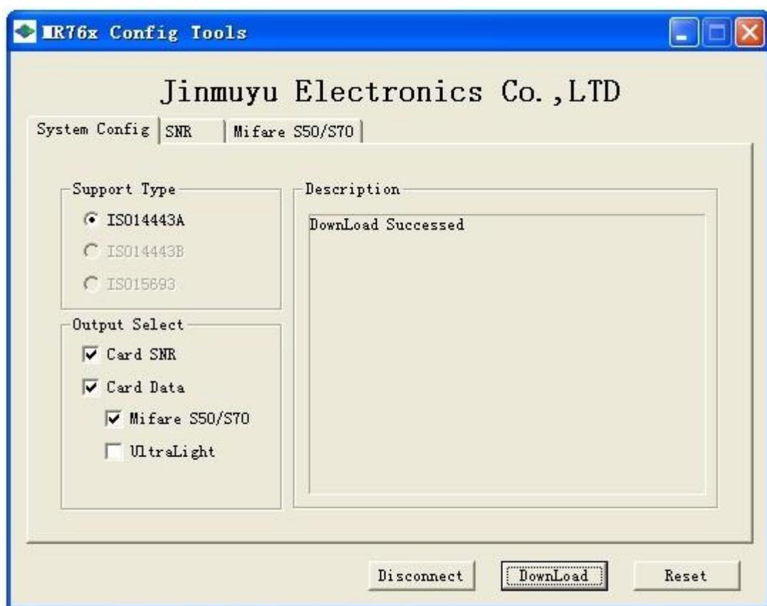
If download success, and then click “Reset” to restart the device. After restart, the computer and device disconnect. Then the computer will re-identify the device and turn to the reading card mode, as following:
